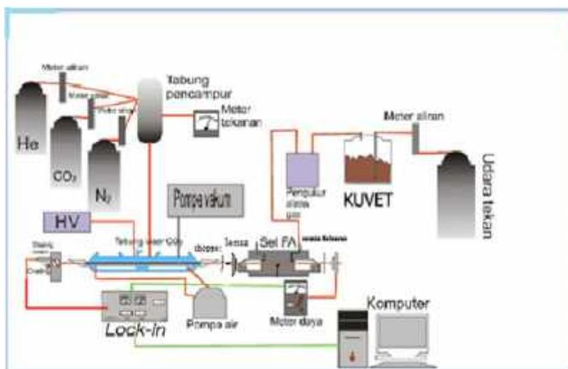
Figure 2.1 Laser  $CO_2$  photoelectric spectroscopy kit
