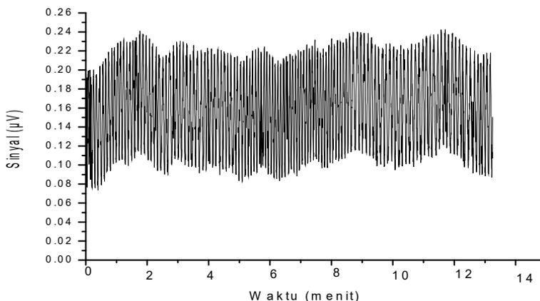
Figure 3.1 CO<sub>2</sub> laser noise
