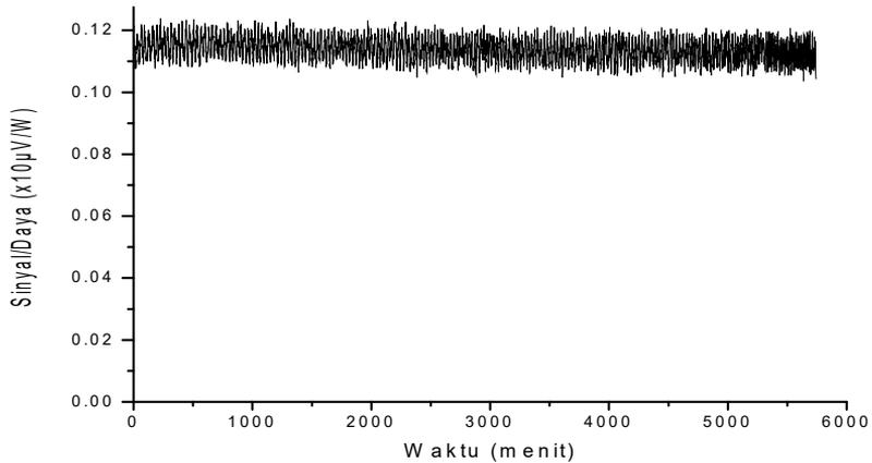
Figure 3.2 CO<sub>2</sub> laser background signal.
