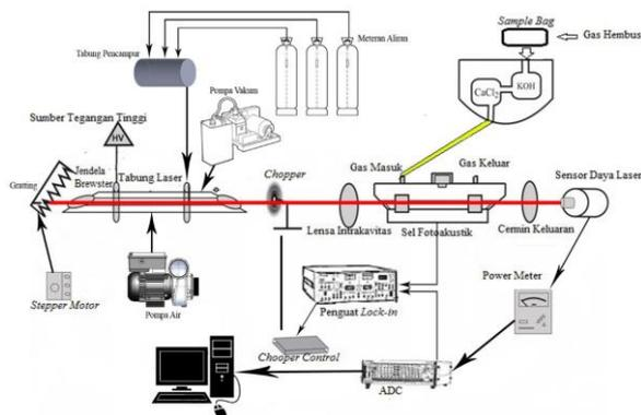
**Figure 3.1 Schematic experimental setup in the study using a CO<sub>2</sub> laser photoacoustic spectrometer intrakavitasi**
