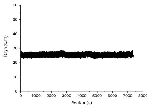
**Figure 4.2. CO<sub>2</sub> laser power stability on the line 10R14**
