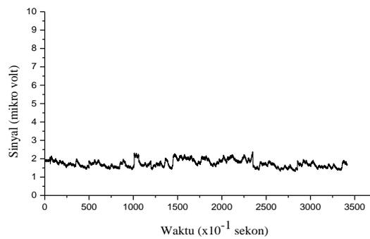
**Figure 4.5. Signal noise photoacoustic cell**
