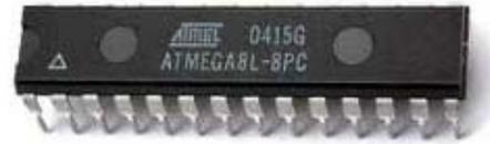
Gambar 3. *ATmega8L 28-pin DIP*
